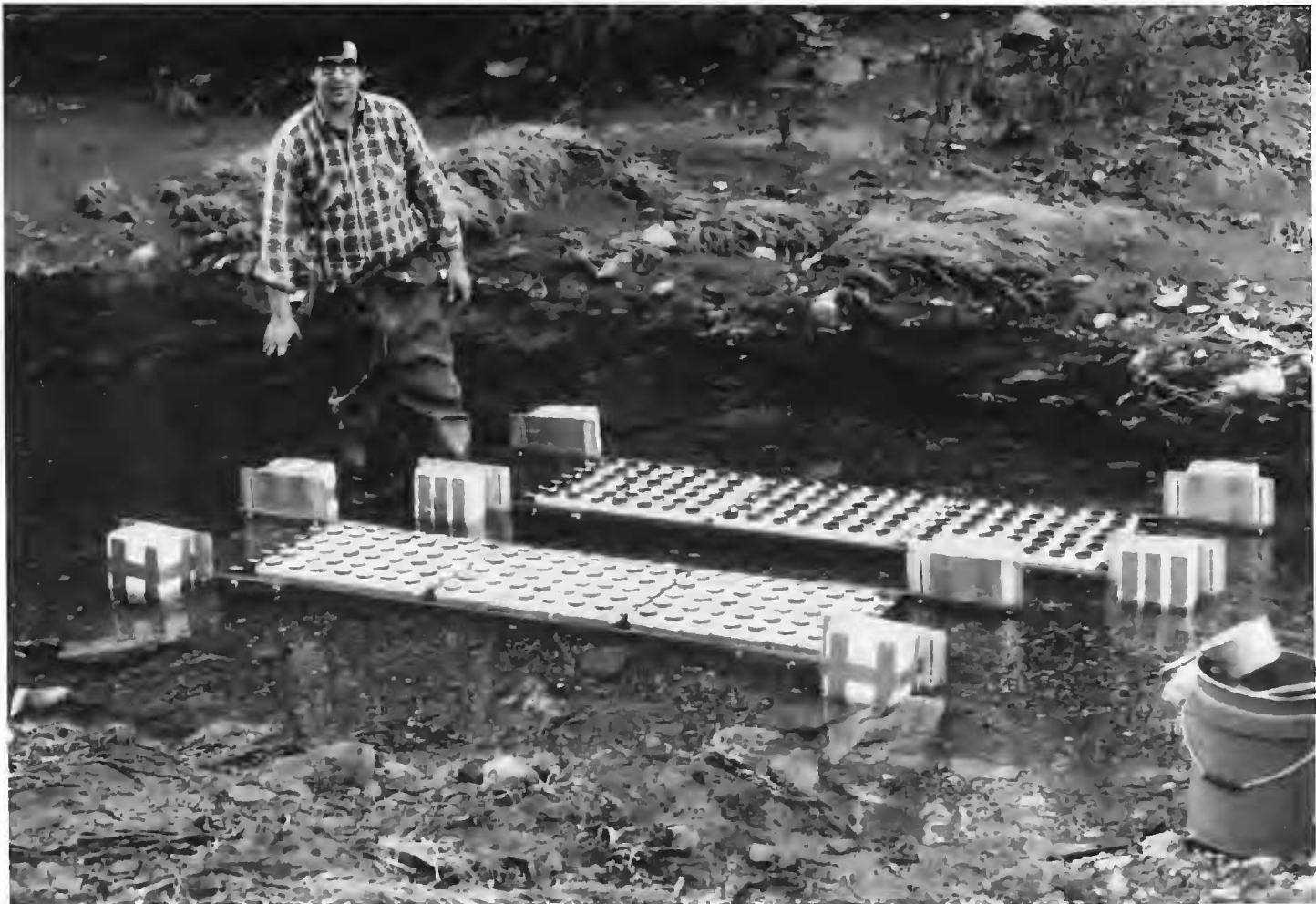
Figure 1. Floating racks used to hold test cells and monitor effects of thermal-shock on stream macroinvertebrates in Big Sulphur Creek, The Geysers, Sonoma Co., California.
